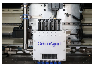
单箱可搭载12种不同规格冲刀 Each toolbox can accommodate up to 12 different punch tools
